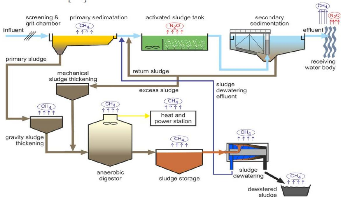
Figure 11. Schematic representation of an activated sludge / anaerobic digestion WWTP shows sources of fugitive emissions of methane and nitrous oxide<sup>5</sup>
