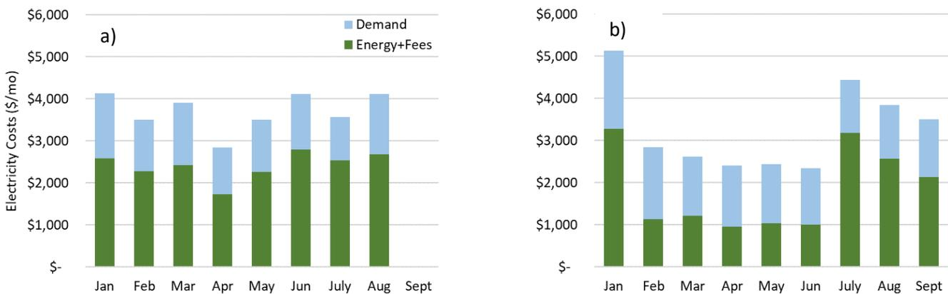
Figure 6. Electricity costs for the (a) wastewater and (b) water treatment plants suggest high fees for power demand (2020)
